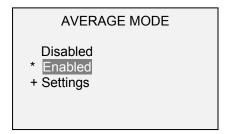
Then, scroll to **Settings**, and press **ENTER** to configure the parameters. The parameters are as follows:
