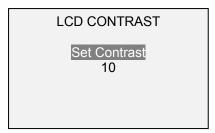
Press ENTER to modify the contrast. Select a value from 0 to 25, 25 producing the most contrast.
