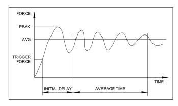
Average mode is used to obtain an average force reading over a specified period of time. This reading also represents the kinetic coefficient of friction for the M5-2-COF gauge. Applications include measurement of peel force, COF, muscle strength, frictional force, and other tests requiring time-averaged readings.
